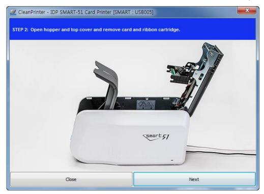
Figure 95 Printer cleaning Step 2
