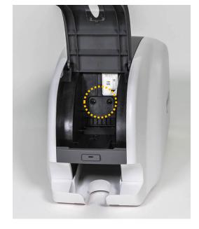
Figure 18 Adjusting the card thickness Device
