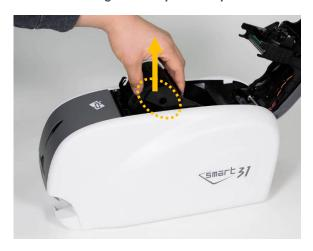
Figure 11 Take out the ribbon cartridge
