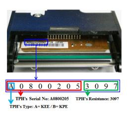
Figure 100 Thermal Print Head
