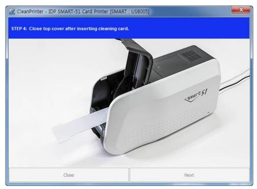
Figure 97 Printer cleaning Step 4
